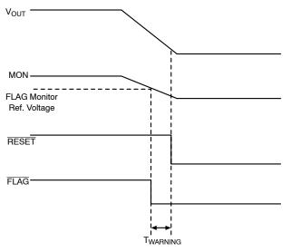
Figure 17. FLAG Monitor Circuit Waveform
