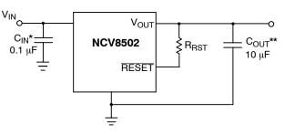
\*C<sub>IN</sub> required if regulator is located far from the power supply filter \*\*C<sub>OUT</sub> required for stability. Capacitor must operate at minimum temperature expected
