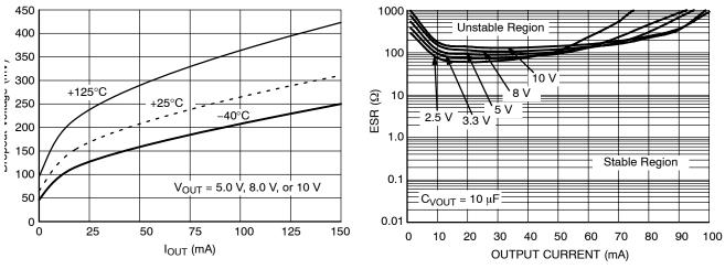
Figure 8. Dropout Voltage vs. Output Current
