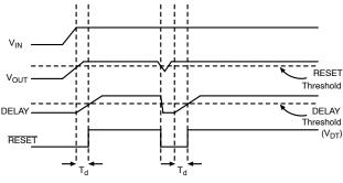
Figure 12. Reset and Delay Circuit Wave Forms
