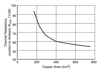
Figure 20. 16 Lead SOW (Exposed Pad), θJA as a Function of the Pad Copper Area (2 oz. Cu Thickness), Board Material = 0.0625″ G-10/R-4
