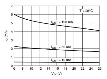
Figure 6. Quiescent Current vs. Input Voltage
