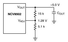
Figure 15. Adjustable Output Voltage
