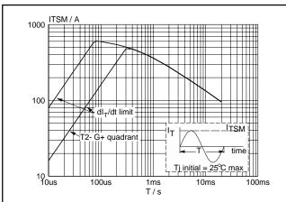
Fig.2. Maximum permissible non-repetitive peak on-state current  $I_{TSM}$ , versus pulse width  $t_p$ , for sinusoidal currents,  $t_p \le 20$ ms.
