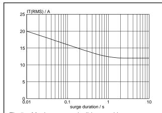
Fig.5. Maximum permissible repetitive rms on-state current  $I_{T(RMS)}$ , versus surge duration, for sinusoidal currents, f = 50 Hz;  $T_{mb} \le 99$ °C.
