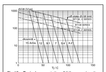
Fig.12. Typical commutation dV/dt versus junction temperature, parameter commutation dl<sub>T</sub>/dt. The triac should commutate when the dV/dt is below the value on the appropriate curve for pre-commutation dl<sub>T</sub>/dt.
