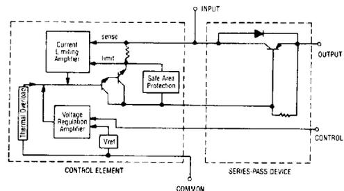
temperature stable band gap reference is the key design factor insuring excellent temperature regulation of the LAS 79HG. This, coupled to a very low output impedance, insures superior load regulation.
