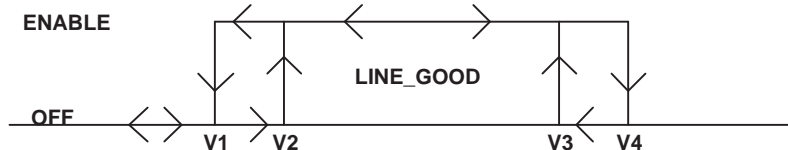
Figure 2. Line UVLO and OVLO Operation
