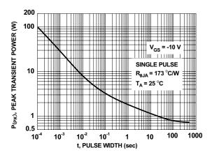
Figure 12. Single Pulse Maximum Power Dissipation
