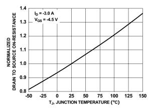
Figure 3. Normalized On-Resistance vs Junction Temperature
