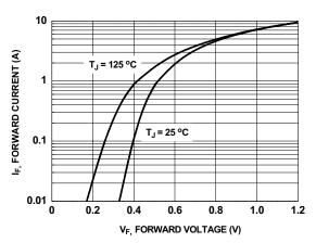
Figure 10. Schottky Diode Foward Voltage
