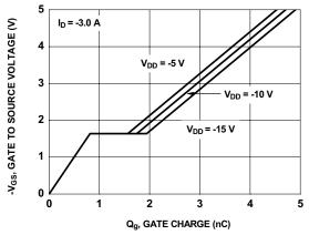
Figure 7. Gate Charge Characteristics
