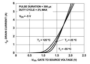
Figure 5. Transfer Characteristics
