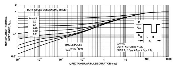
Figure 13. Junction to Ambient Transient Thermal Response Curve
