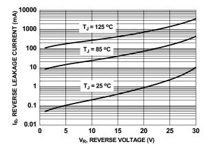
Figure 11. Schottky Diode Reverse Current
