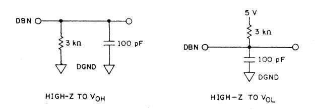
FIGURE 5. Load circuits for data access time.
