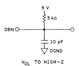
FIGURE 4. Load circuits for data hold time.
