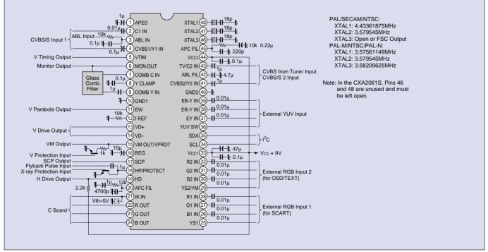
■ Figure 2 CXA2060AS/CXA2061S Application Circuit Example
