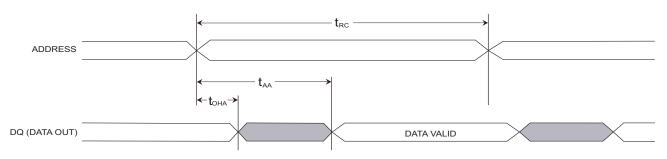
Figure 6. SRAM Read Cycle 2:  $\overline{CE}$  and  $\overline{OE}$  Controlled <sup>[7, 10]</sup>
