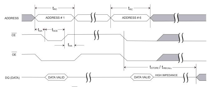
Figure 11. OE Controlled Software STORE/RECALL Cycle [17]
