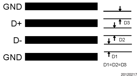
FIGURE 4. Ideal Diode Trace Layout
