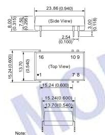
Pin section: 0.60\*0.25mm(0.024\*0.010inch) Pin tolerances: ±0.10mm(±0.004inch)
