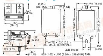
Note: The 263/268 Series Relay is a 15 Amp Version of the 262/267 Series Relay Except With .187" Quick Connect Terminals. The User May Utilize the 260 Series Dimensions @Rage 15 for Further Detail.
