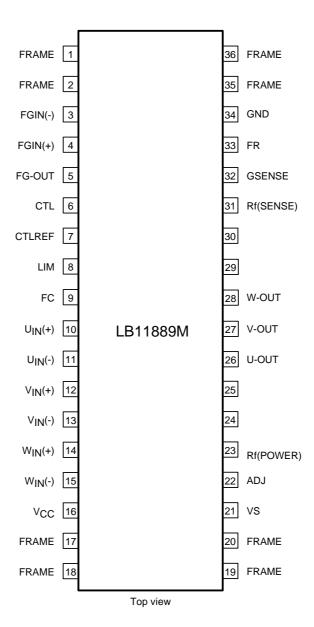
Note: Although the FRAME pins and the GND pin are not connected internally in the IC, the FRAME pins must be connected to the GND pin externally for ground potential stabilization.
