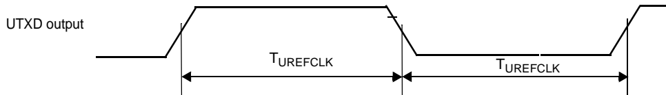
Figure 22. UART Output Timing
