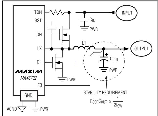
Figure 8. Standard Application with Output Polymer or Tantalum
