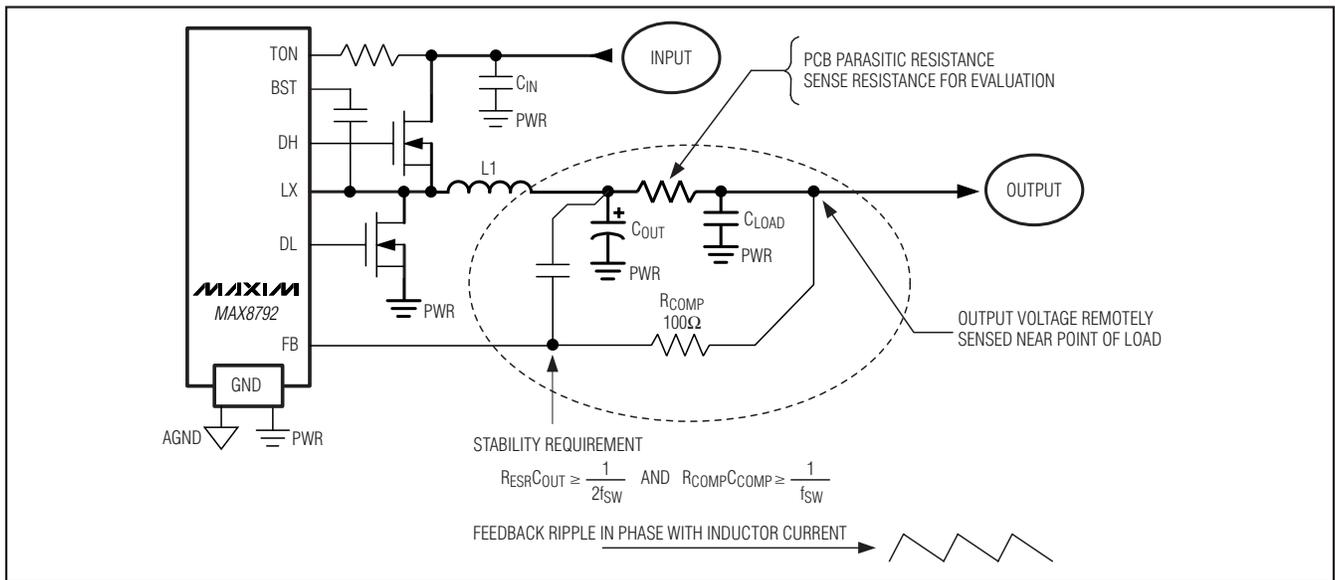
Figure 9. Remote-Sense Compensation for Stability and Noise Immunity
