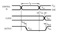
FIGURE 5. Propagation Delay, Pulse Width and  $$t_{\rm rec}$$  Waveforms
