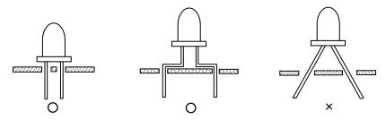
3-2) Therefore please design holes of PCB suitable for termination space or termination space after forming, and avoid the stress.
