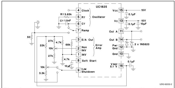
This test fixture is useful for exercising many of the As with any wideband circuit, careful grounding and by-UC1825's functions and measuring their specifications.
