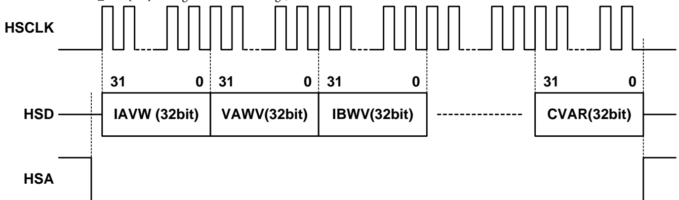
Figure 66. HSDC communication for HGAP=0, HXFER[1:0]=00 and HSAPOL=0. HSIZE is irrelevant
