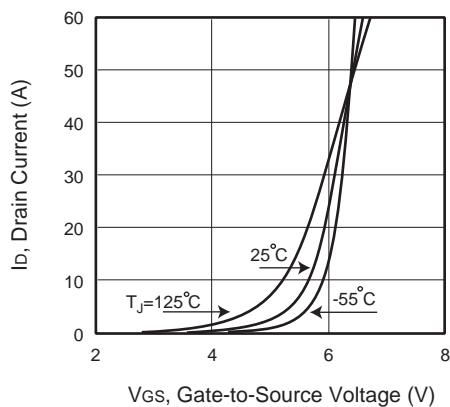
Figure 2. Transfer Characteristics
