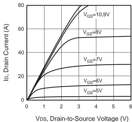
Figure 1. Output Characteristics
