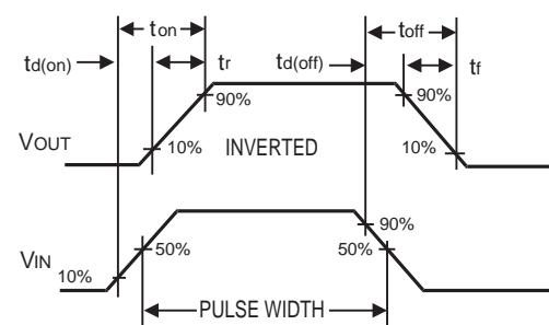
Figure 10. Switching Waveforms
