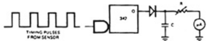
C and R determines the meter reading for a given input pulse rate. R may be used to calibrate the meter to show rpm or other rate of the equipment being monitored.
