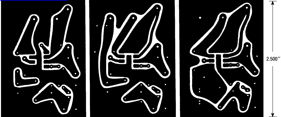
(Top view, copper foil as seen through the board from the component side)
