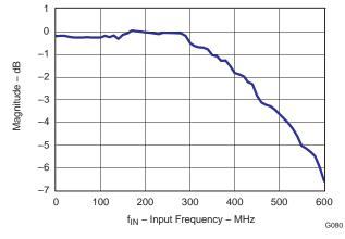
Figure 90. ADC Analog Input Bandwidth
