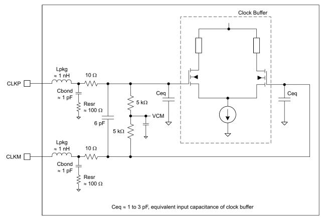
Figure 97. Internal Clock Buffer
