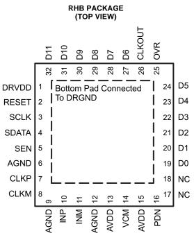
Figure 7. CMOS Mode Pinout
