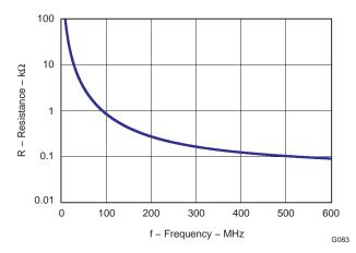
Figure 91. ADC Input Resistance, Rin
