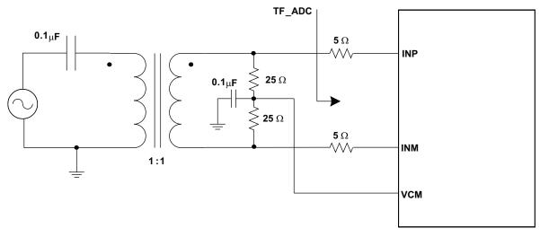
Figure 93. Single Transformer Drive Circuit
