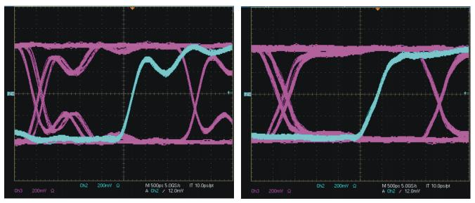
Figure 104. LVDS Eye Diagram - No Internal Termination 5-pF Load Capacitance Blue Trace - Output Clock (CLKOUT) Pink Trace - Output Data
