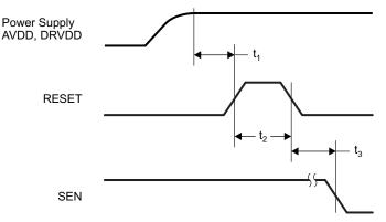
NOTE: A high-going pulse on RESET pin is required in serial interface mode in case of initialization through hardware reset. For parallel interface operation, RESET has to be tied permanently HIGH.
