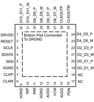
Figure 8. LVDS Mode Pinout
