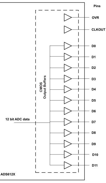
Figure 101. CMOS Output buffers
