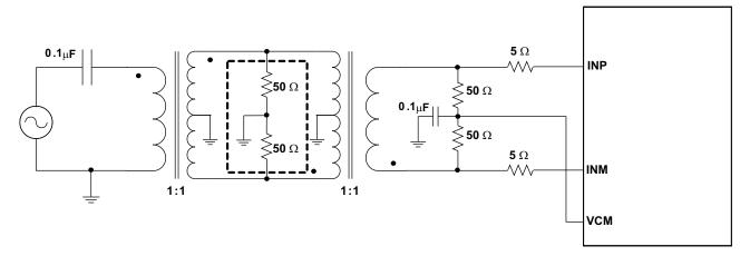
Figure 94. Two Transformer Drive Circuit
