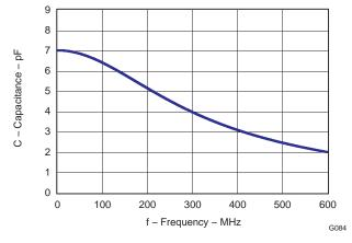
Figure 92. ADC Input Capacitance, Cin
