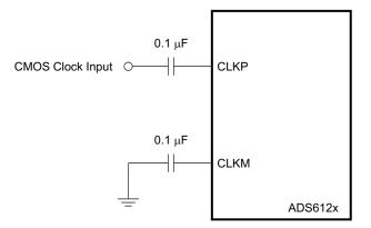
Figure 100. Single-Ended Clock Driving Circuit
