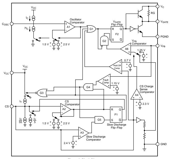
Figure 2. Block Diagram
