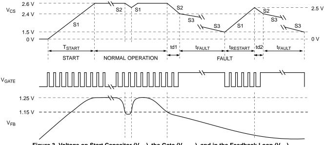
Figure 3. Voltage on Start Capacitor (V<sub>GS</sub>), the Gate (V<sub>GATE</sub>), and in the Feedback Loop (V<sub>FB</sub>), During Startup, Normal and Fault Conditions
