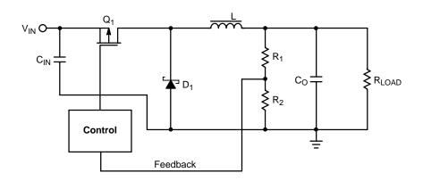
Figure 4. Buck Regulator Block Diagram
