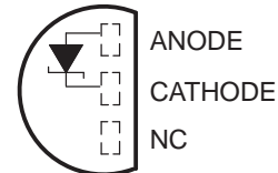
LP (TO-92/TO-226) PACKAGE (TOP VIEW)
