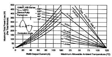
Fig. 13 - Total Power Loss Characteristics
