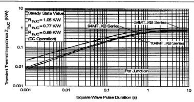
Fig. 16 - Thermal Impedance Z<sub>th/C</sub> Characteristics
