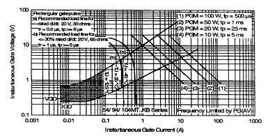
Fig. 17 - Gate Characteristics
