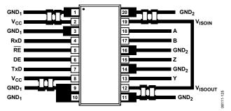
Figure 35. Recommended PCB Layout
