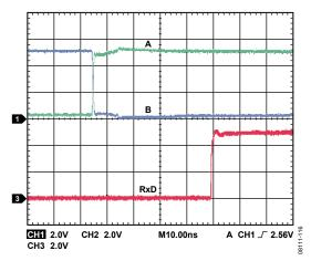
Figure 16. ADM2587E Receiver Propagation Delay
