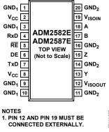
Figure 2. Pin Configuration
