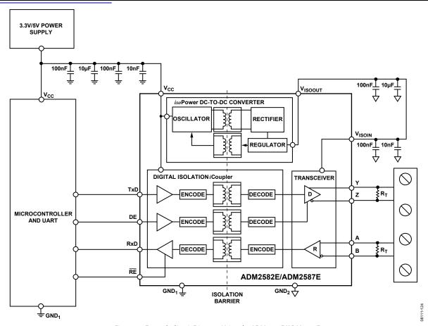
Figure 40. Example Circuit Diagram Using the ADM2582E/ADM2587E
