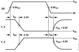
Figure 31. Driver Enable/Disable Timing
