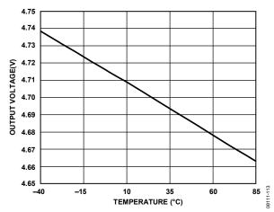
Figure 13. Receiver Output High Voltage vs. Temperature
