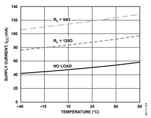
Figure 4. ADM2582E Supply Current (lcc) vs. Temperature (Data Rate = 16 Mbps, DE = 5 V, Vcc = 5 V)
