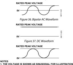
THE LIMITING VALUE CAN BE POSITIVE OR NEGATIVE, BUT THE Figure 38. Unipolar AC Waveform
