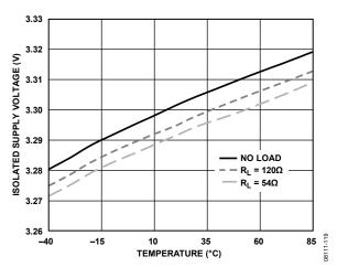
Figure 19. ADM2582E Isolated Supply Voltage vs. Temperature  $(V_{CC} = 3.3 \text{ V}, Data Rate = 16 \text{ Mbps})$
