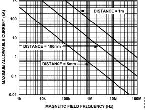
Figure 34. Maximum Allowable Current for Various Current-to-ADM2582E/ADM2587E Spacings
