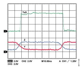
Figure 9. ADM2582E Driver Propagation Delay
