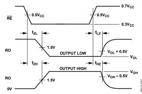
Figure 32. Receiver Enable/Disable Timing
