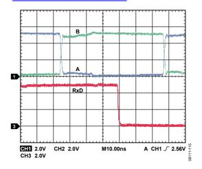
Figure 15. ADM2582E Receiver Propagation Delay
