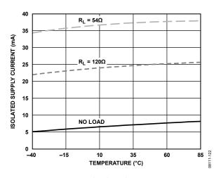
Figure 22. ADM2587E Isolated Supply Current vs. Temperature  $(V_{CC} = 3.3 V, Data Rate = 500 kbps)$
