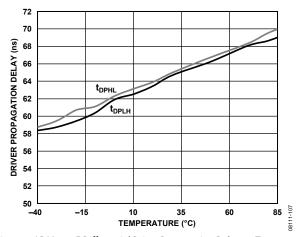
Figure 7. ADM2582E Differential Driver Propagation Delay vs. Temperature
