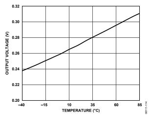
Figure 14. Receiver Output Low Voltage vs. Temperature
