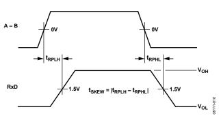
Figure 30. Receiver Propagation Delay
