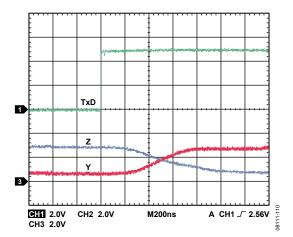
Figure 10. ADM2587E Driver Propagation Delay
