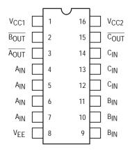
Pin assignment is for Dual–in–Line Package.
