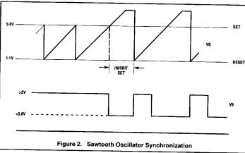
Synchronization at a frequency lower than the free-running frequency is accomplished via the TTL gate on Pin 9. By activating this gate ( $V^9 < 2V$ ), the setting of the sawtooth is prevented. This is indicated in Figure 2.
