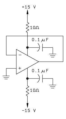
FIGURE 2. Radiation exposure circuit.
