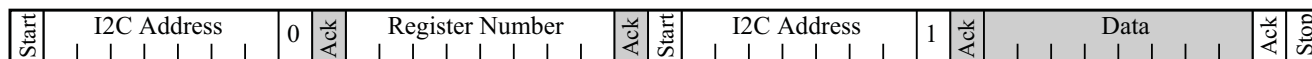
Figure 29. Format of a Register Read. Shaded Regions Denote Bus Control by TPS2358/9
