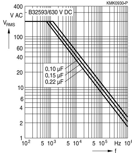
**Permissible AC voltage  $V_{\text{RMS}}$  versus frequency  $f$  (for sinusoidal waveforms,  $T_A \leq 55^\circ\text{C}$ )**
