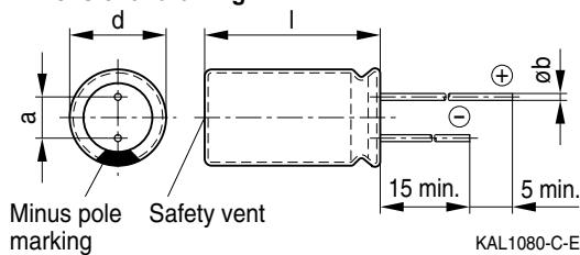
Safety vent for diameter  $\geq 8$  mm.
