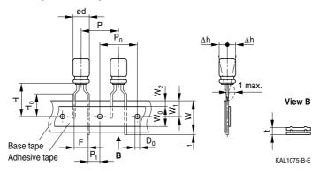
Lead spacing 5.0 mm ( $\varnothing$  d = 10 mm)
