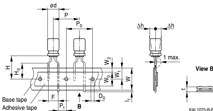
**Lead spacing 5.0 mm ( $\varnothing d = 10 \text{ mm}$ )**
