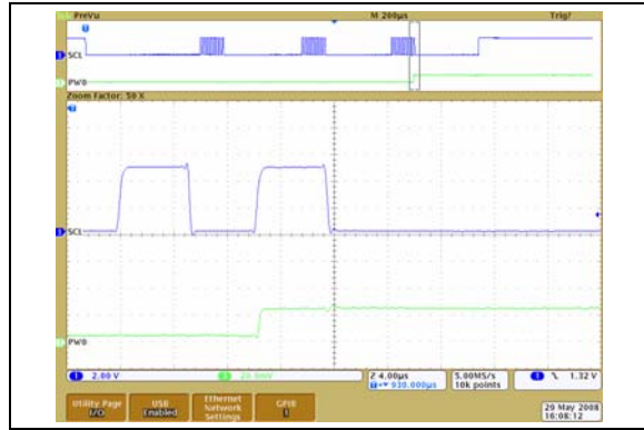
FIGURE 2-43: 50 k \Omega – Low-Voltage Increment Wiper Settling Time ( V_{DD} = 5.5\text{V} ) (1 \mu\text{s}/\text{Div} ).
