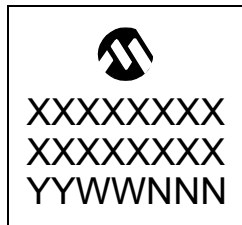
28-Lead QFN (6mm x 6mm)
