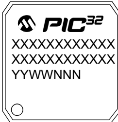
100-Lead TQFP (14x14x1 mm)
