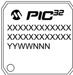
100-Lead TQFP (12x12x1 mm)
