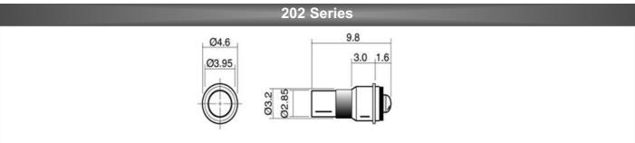
Dimensions in mm (Typical) Not to scale Green dot on base of product signifies centre contact cathode -ve. Colour sleeve on product denotes LED colour.
