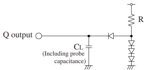
$$\begin{aligned} C_L &= 15\text{pF} : \text{DUTY}, I_{DD}, t_{r3}, t_{f3} \\ C_L &= 50\text{pF} : t_{r5}, t_{f5} \\ R &= 400\Omega \end{aligned}$$
