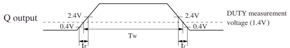
**Output duty cycle (CMOS)**
