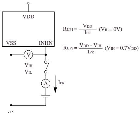
$$R_{UP1} = \frac{V_{DD}}{I_{PR}} \quad (V_{IL} = 0V)$$
