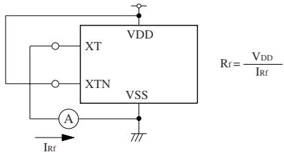
$$R_f = \frac{V_{DD}}{I_{rf}}$$
