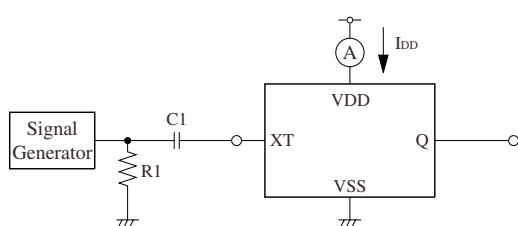
2.0V<sub>P-P</sub>, 30MHz sine wave input signal (3V operation)
