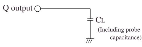
$$\begin{aligned} C_L &= 15\text{pF} : \text{DUTY}, I_{DD}, t_{r1}, t_{f1} \\ C_L &= 30\text{pF} : t_{r4}, t_{f4} \\ C_L &= 50\text{pF} : t_{r2}, t_{f2} \end{aligned}$$
