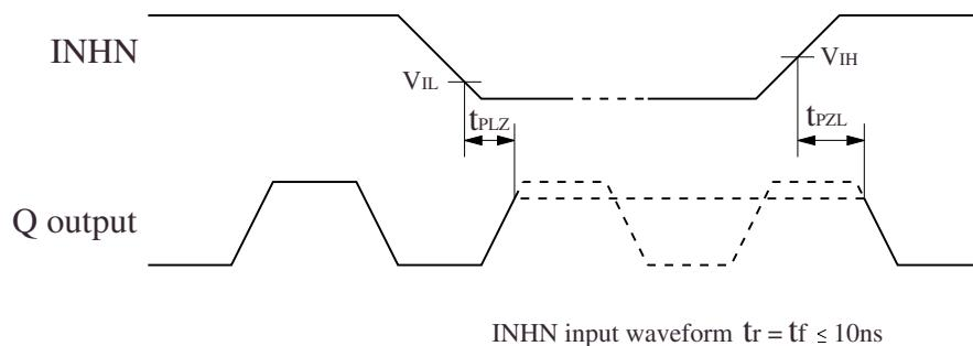
Note (CL $\times$ /EA $\times$  series only): when the device is in standby, the oscillator stops. When standby is released, the oscillator starts and stable oscillator output occurs after a short delay.
