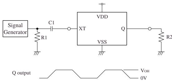
2.0V<sub>P-P</sub>, 10MHz sine wave input signal (3V operation)
