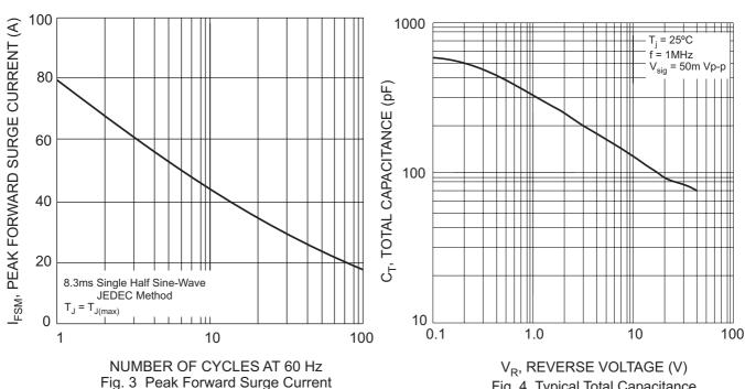
Fig. 4 Typical Total Capacitance
