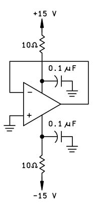
FIGURE 2. Radiation exposure circuit.
