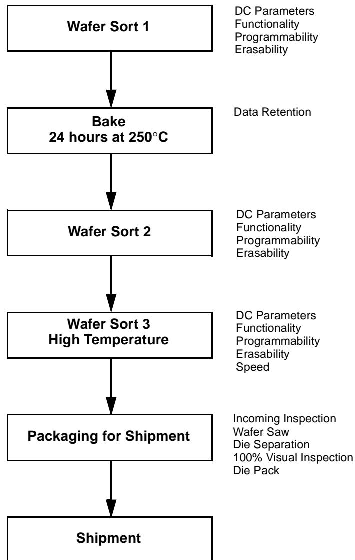
Figure 1. AMD KGD Product Test Flow
