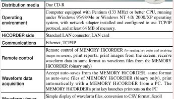
function, enlarge/reduce display, display CH settings.
