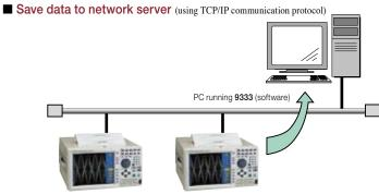
Copy measurement data files obtained from HiCORDER to PC on network
