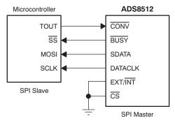
NOTE: CPOL = 0 (inactive SCLK is LOW) CPHA = 0 or 1 (data valid on either SCLK edge)
