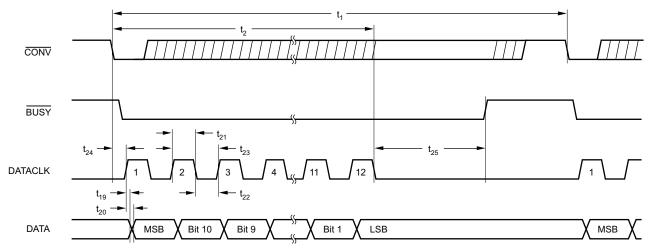
Figure 43. Serial Data Timing, External Clock, Clocking During the Next Conversion (EXT/INT High, CS Low)
