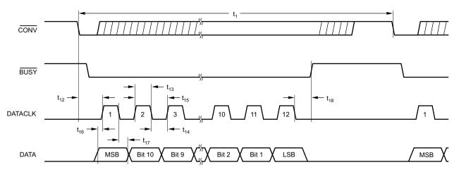
Figure 40. Serial Data Timing, Internal Clock (EXT/INT and CS Low)
