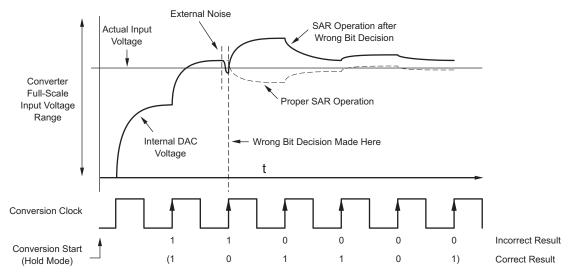
Figure 50. SAR Operation When External Noise Affects the Conversion
