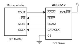
NOTE: CPOL = 0 (inactive SCLK is LOW) CPHA = 1 (data valid on SCLK falling edge)
