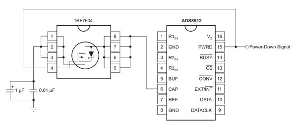
Figure 49. Improved Power-Up Response Circuit
