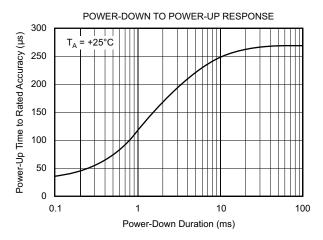
Figure 48. Power-Down to Power-Up Response
