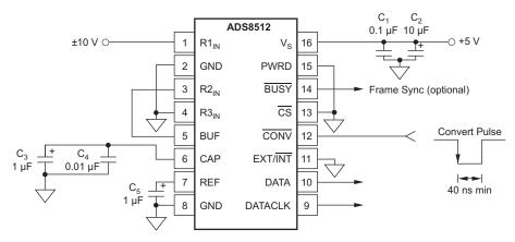
Figure 36. Basic Operating Circuit, ±10-V Input Range, Internal DATACLK
