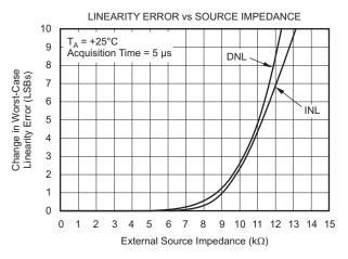
Figure 47. Linearity Error vs Source Impedance in High Impedance Mode (R1<sub>IN</sub> = R2<sub>IN</sub> = R3<sub>IN</sub> = V<sub>IN</sub>)
