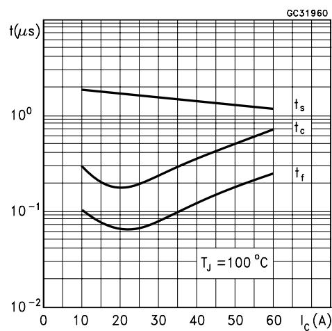
Switching Times Inductive Load Versus Temperature
