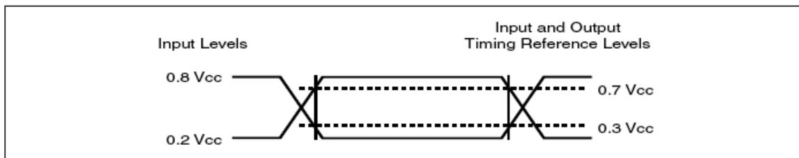
Figure 22. AC Measurement I/O Waveform
