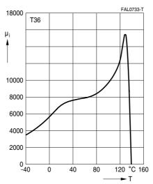
Variation of initial permeability with temperature (measured on R22 toroids,  $\hat{B} \le 0.25$  mT)
