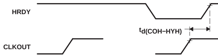
Figure 39. \text{HRDY} Relative to \text{CLKOUT}
