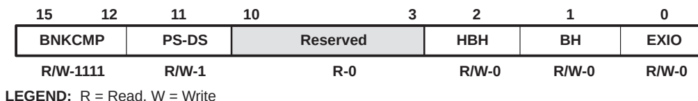
Figure 5. Bank-Switching Control Register (BSCR) [MMR Address 0029h]
