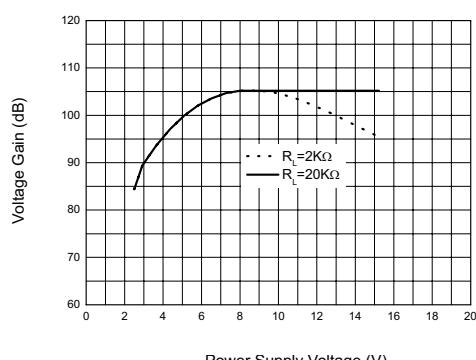
Figure 7. Voltage Gain
