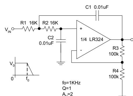
Figure 21. DC Coupled Low-Pass RC Active Filter
